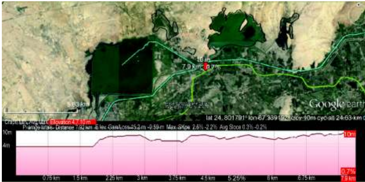
Fig. 5. Elevation profile of Jamwah Canal feeding Haleji Lake.
