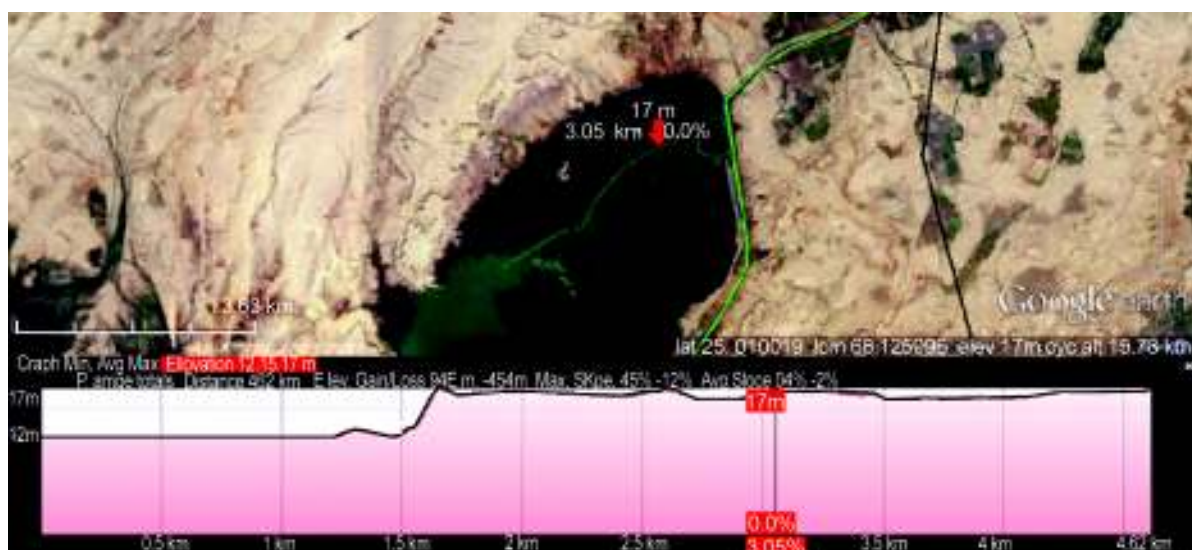
Fig. 4. Elevation profile canal feeding Keenjhar
